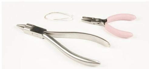
Snipping pliers, needle nose pliers and flat nose pliers, a stronger wire with a diameter of about 1 mm or skewers (they are used for twisting the wire)
