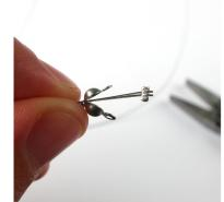
3) Move the crimp bead to the end of both wires and then squeeze it with flatnose pliers, so it becomes flat.
